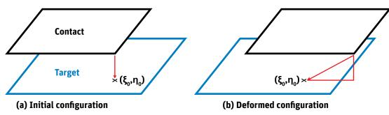
Gap and slip are measured from the contact detection point to its original nature coordinator of intersection on target.
