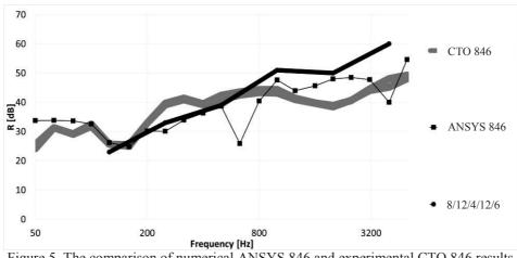
Figure 5. The comparison of numerical ANSYS 846 and experimental CTO 846 results for 8/12/4/12/6 type of window glazing
