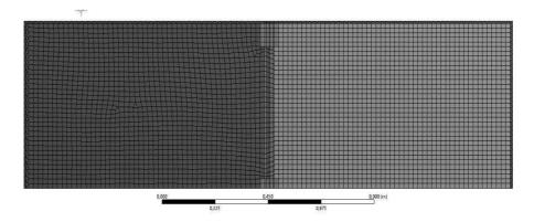
Figure 3. Geometry of the model (half-bottom view) and finite element size
